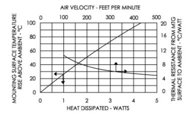
\*Natural convection thermal resistance is based on a 75 °C heat sink temperature rise.
